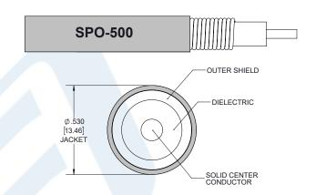
ing SPO-500 Coax Using Times Microwave Parts PE3C6373-24
