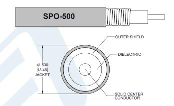
ing SPO-500 Coax Using Times Microwave Parts PE3C6373-150CM
