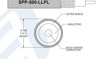
Click the following link (or enter part number in "SEARCH" on website) to obtain additional part information including price, inventory and certifications: Plenum N Male to N Male Low PIM Cable 48 Inch Length Using SPP-500-LLPL Coax Using Times Microwave Parts PE3C6370-48
