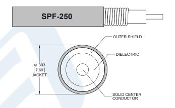
inventory and certifications: Fire Rated N Male to NEX10 Male Low PIM Cable 48 Inch Length Using SPF-250 Coax Using Times Microwave Parts PE3C6362-48
