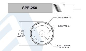
SPF-250 Coax Using Times Microwave Parts PE3C6359-48
