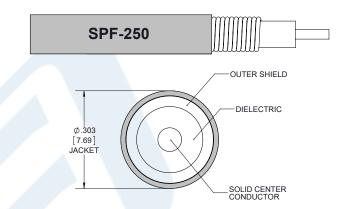
SPF-250 Coax Using Times Microwave Parts PE3C6359-36
