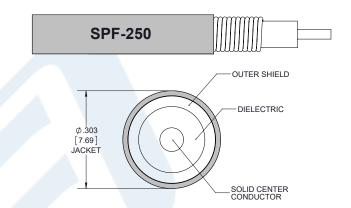
inventory and certifications: Fire Rated 7/16 DIN Male to N Male Low PIM Cable 12 Inch Length Using SPF-250 Coax Using Times Microwave Parts PE3C6357-12
