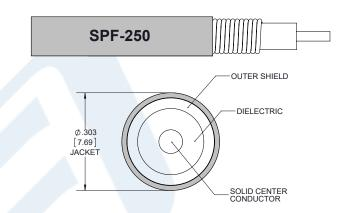
price, inventory and certifications: Fire Rated 7/16 DIN Male to 7/16 DIN Male Low PIM Cable 24 Inch Length Using SPF-250 Coax Using Times Microwave Parts PE3C6356-24
