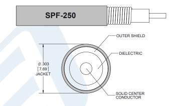
SPF-250 Coax Using Times Microwave Parts PE3C6356-12
