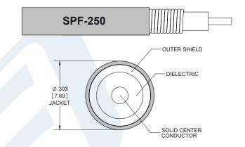
SPF-250 Coax Using Times Microwave Parts PE3C6356-100CM
