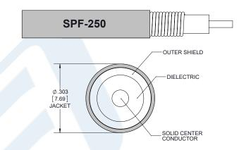
SPF-250 Coax Using Times Microwave Parts PE3C6355-36
