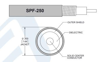
SPF-250 Coax Using Times Microwave Parts PE3C6355-150CM
