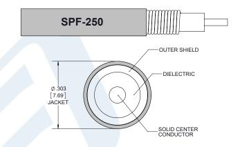
Using SPF-250 Coax Using Times Microwave Parts PE3C6354-12
