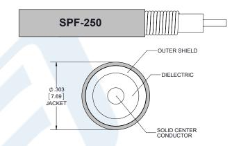
SPF-250 Coax Using Times Microwave Parts PE3C6352-200CM
