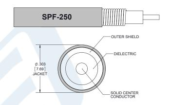
price, inventory and certifications: Fire Rated 4.3-10 Female to 4.3-10 Female Low PIM Cable 36 Inch Length Using SPF-250 Coax Using Times Microwave Parts PE3C6348-36
