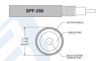
SPF-250 Coax Using Times Microwave Parts PE3C6348-150CM
