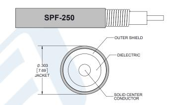
SPF-250 Coax Using Times Microwave Parts PE3C6348-12
