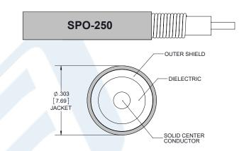
SPO-250 Coax Using Times Microwave Parts PE3C6344-200CM
