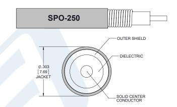
SPO-250 Coax Using Times Microwave Parts PE3C6344-150CM
