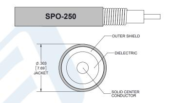
SPO-250 Coax Using Times Microwave Parts PE3C6343-100CM
