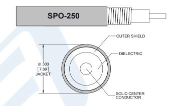
ing SPO-250 Coax Using Times Microwave Parts PE3C6340-60
