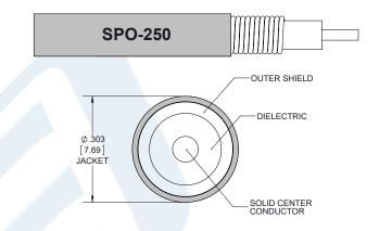
ing SPO-250 Coax Using Times Microwave Parts PE3C6340-200CM
