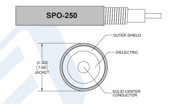
ing SPO-250 Coax Using Times Microwave Parts PE3C6340-12
