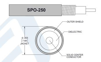
Length Using SPO-250 Coax Using Times Microwave Parts PE3C6339-12
