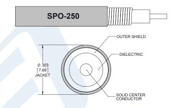
SPO-250 Coax Using Times Microwave Parts PE3C6337-36
