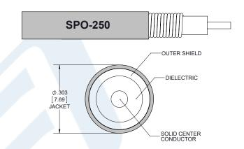
SPO-250 Coax Using Times Microwave Parts PE3C6337-150CM
