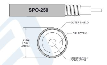
Using Times Microwave Parts PE3C6336-200CM
