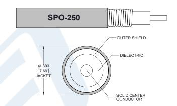
SPO-250 Coax Using Times Microwave Parts PE3C6332-50CM
