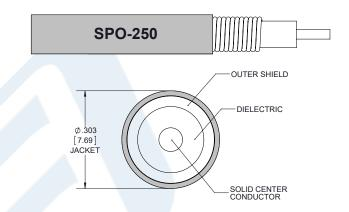
ing SPO-250 Coax Using Times Microwave Parts PE3C6332-48
