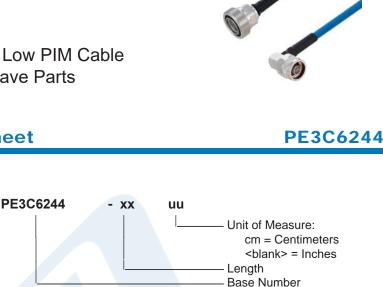
Example: PE3C6244-12 = 12 inches long cable PE3C6244-100cm = 100 cm long cable
