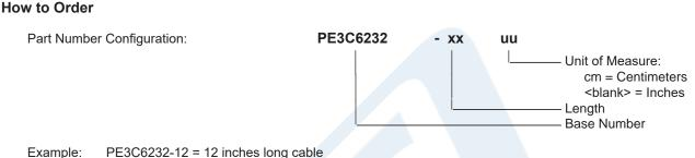
ple: PE3C6232-12 = 12 inches long cable PE3C6232-100cm = 100 cm long cable
