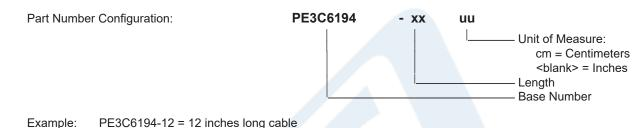
Plenum 7/16 DIN Male to SMA Male Low PIM Cable 12 Inch Length Using SPP-250-LLPL Coax Using Times Microwave Parts from Pasternack Enterprises has same day shipment for domestic and International orders. Our RF, microwave and millimeter wave products maintain a 99.4% availability and are part of the broadest selection in the industry.
