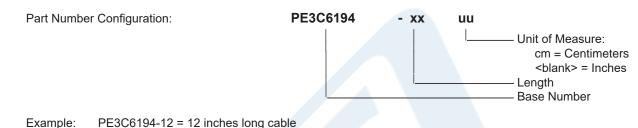
Plenum 7/16 DIN Male to SMA Male Low PIM Cable 100 cm Length Using SPP-250-LLPL Coax Using Times Microwave Parts from Pasternack Enterprises has same day shipment for domestic and International orders. Our RF, microwave and millimeter wave products maintain a 99.4% availability and are part of the broadest selection in the industry.
