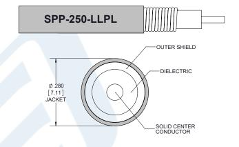
Click the following link (or enter part number in "SEARCH" on website) to obtain additional part information including price, inventory and certifications: Plenum SMA Male Right Angle to SMA Male Right Angle Low PIM Cable 36 Inch Length Using SPP-250-LLPL Coax , LF Solder PE3C5895-36
