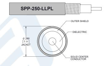
Click the following link (or enter part number in "SEARCH" on website) to obtain additional part information including price, inventory and certifications: Plenum SMA Male Right Angle to SMA Male Right Angle Low PIM Cable 12 Inch Length Using SPP-250-LLPL Coax , LF Solder PE3C5895-12
