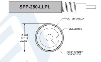
Click the following link (or enter part number in "SEARCH" on website) to obtain additional part information including price, inventory and certifications: Plenum 7/16 DIN Male to SMA Female Low PIM Cable 48 Inch Length Using SPP-250-LLPL Coax , LF Solder PE3C5880-48
