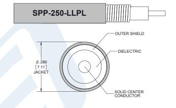
Click the following link (or enter part number in "SEARCH" on website) to obtain additional part information including price, inventory and certifications: Plenum 7/16 DIN Male to SMA Female Low PIM Cable 100 cm Length Using SPP-250-LLPL Coax, LF Solder PE3C5880-100CM
