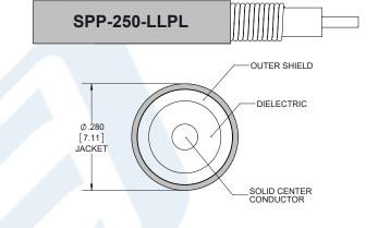
Click the following link (or enter part number in "SEARCH" on website) to obtain additional part information including price, inventory and certifications: Plenum QMA Male Right Angle to QMA Male Right Angle Low PIM Cable 24 Inch Length Using SPP-250-LLPL Coax, LF Solder PE3C5877-24
