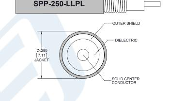
Click the following link (or enter part number in "SEARCH" on website) to obtain additional part information including price, inventory and certifications: Plenum 4.1/9.5 Mini DIN Male Right Angle to N Male Low PIM Cable 12 Inch Length Using SPP-250-LLPL Coax , LF Solder PE3C5849-12
