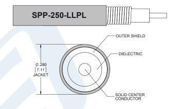
Click the following link (or enter part number in "SEARCH" on website) to obtain additional part information including price, inventory and certifications: Plenum 4.1/9.5 Mini DIN Female to QMA Male Low PIM Cable 12 Inch Length Using SPP-250-LLPL Coax , LF Solder PE3C5844-12
