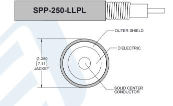
Click the following link (or enter part number in "SEARCH" on website) to obtain additional part information including price, inventory and certifications: Plenum 4.1/9.5 Mini DIN Female to N Male Low PIM Cable 100 cm Length Using SPP-250-LLPL Coax , LF Solder PE3C5843-100CM
