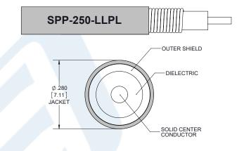
Click the following link (or enter part number in "SEARCH" on website) to obtain additional part information including price, inventory and certifications: Plenum 4.1/9.5 Mini DIN Female to 7/16 DIN Male Low PIM Cable 60 Inch Length Using SPP-250-LLPL Coax , LF Solder PE3C5842-60
