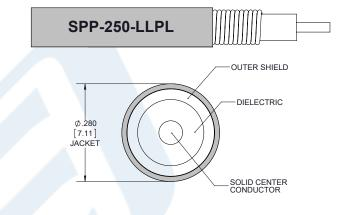
Click the following link (or enter part number in "SEARCH" on website) to obtain additional part information including price, inventory and certifications: Plenum 4.1/9.5 Mini DIN Female to 7/16 DIN Male Low PIM Cable 48 Inch Length Using SPP-250-LLPL Coax , LF Solder PE3C5842-48
