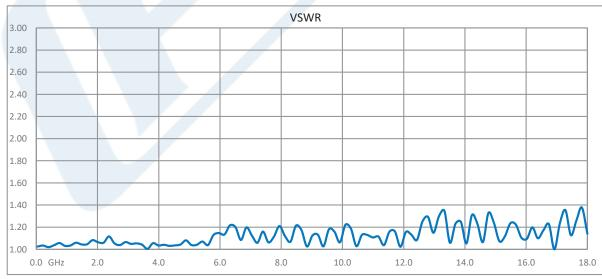
Click the following link (or enter part number in "SEARCH" on website) to obtain additional part information including price, inventory and certifications: N Female Bulkhead to SMA Male Low Loss Cable 24 Inch Length Using PE-P160LL Coax PE3C5274-24
