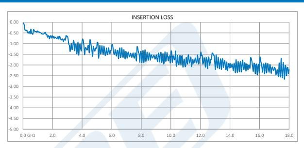
Click the following link (or enter part number in "SEARCH" on website) to obtain additional part information including price, inventory and certifications: SMA Female Bulkhead to TNC Male Right Angle Low Loss Cable 12 Inch Length Using PE-P160LL Coax PE3C5265-12
