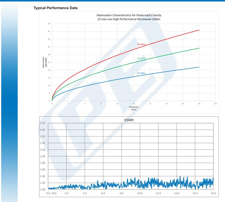
Click the following link (or enter part number in "SEARCH" on website) to obtain additional part information including price, inventory and certifications: SMA Female Bulkhead to TNC Male Low Loss Cable 150 CM Length Using PE-P160LL Coax PE3C5264-150CM
