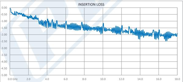
Click the following link (or enter part number in "SEARCH" on website) to obtain additional part information including price, inventory and certifications: SMA Male to TNC Female Bulkhead Low Loss Cable 60 Inch Length Using PE-P160LL Coax PE3C5260-60
