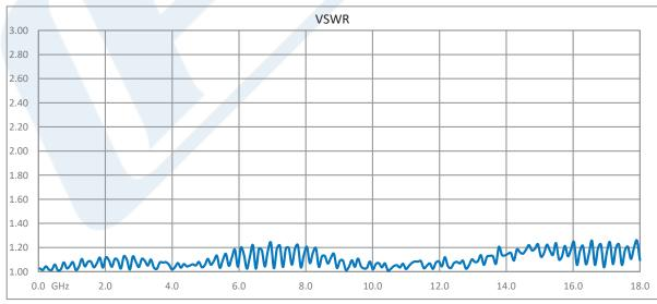
Click the following link (or enter part number in "SEARCH" on website) to obtain additional part information including price, inventory and certifications: N Male to N Female Bulkhead Low Loss Cable 12 Inch Length Using PE-P160LL Coax PE3C5257-12
