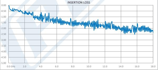
Click the following link (or enter part number in "SEARCH" on website) to obtain additional part information including price, inventory and certifications: N Female Bulkhead to N Female Bulkhead Low Loss Cable 24 Inch Length Using PE-P160LL Coax PE3C5256-24
