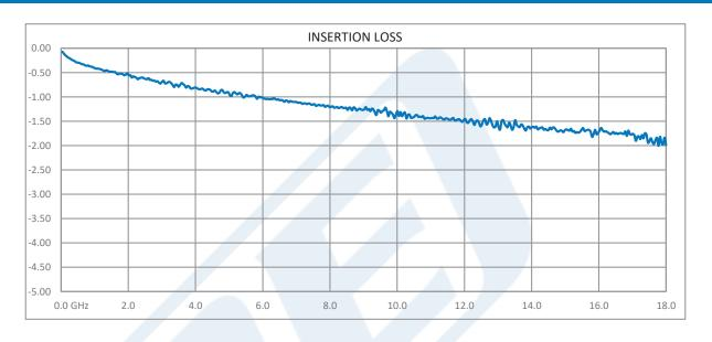
Click the following link (or enter part number in "SEARCH" on website) to obtain additional part information including price, inventory and certifications: SMA Male Right Angle to SMA Male Right Angle Low Loss Cable Using PE-P160LL Coax PE3C5248
